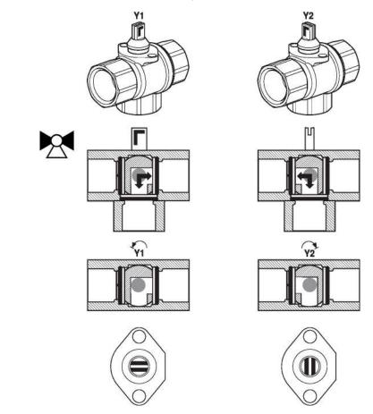
**Flow setting** At the actuator the end stop clip has to be removed in order to get the angle of rotation of 90°, which is needed for the change-over functionality.
