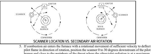
pilot flame in direction of rotation, position the scanner 0 to 30 degrees downstream of the pilot burner and close to the periphery of the throat where the ultraviolet radiation is at a maximum. (See Figures 3 and 4).Having determined an appropriate location for the sight tube, cut a clearance hole for a 2 inch
