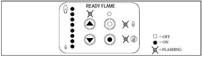
Keeping the target flame button depressed, use the flame strength LEDs to adjust the scanner "aim" to get maximum signal (1 LED is the lowest, 8 LEDs are the highest). Look for 3 to 4 LEDs as a minimum.
