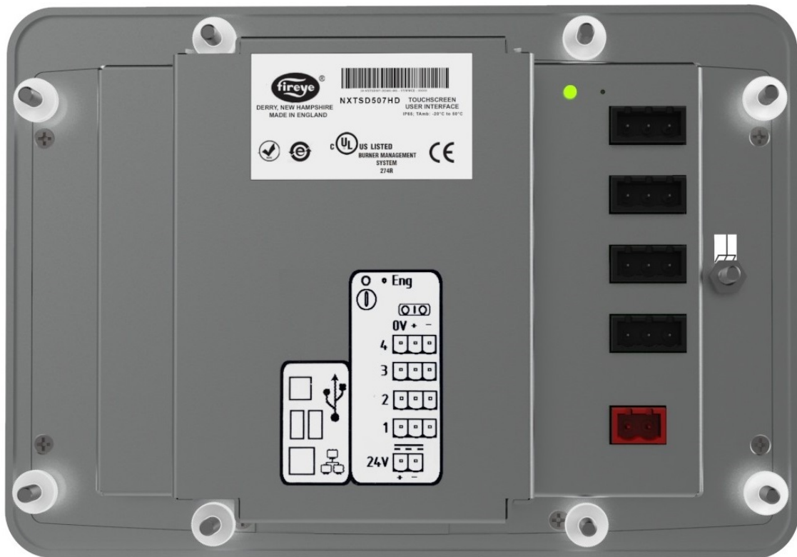
Rear of NXTSD507HD showing placement of the knurled-head thumb nuts
