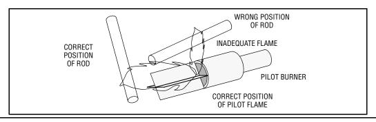
**5.** If the flame is partly luminous, the electrode tip should extend only to the edge of the flame. It is not necessary to maintain absolutely uninterrupted contact with the flame.
