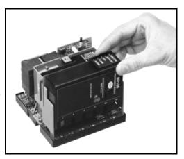
opens, remove the fuse (using a small screwdriver) and install a Fireye replacement fuse (P/N 23-176) or equivalent 2AG, 8 amp fuse (e.g. Littlefuse #225008) In programmers used with the MC230 and MC230R, use replacement fuse P/N 23-183 or equivalent (3.5 amp, 2AG, SLO-BLO) Littlefuse #22903.5.
