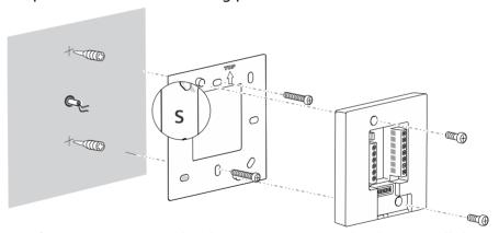
If you are mounting the thermostat on a conduit box, install the metal
