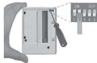
Step 4. Set application DIP switches. See DIP Switch Settings .
