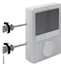
Step 1. Loosen retaining screws.
