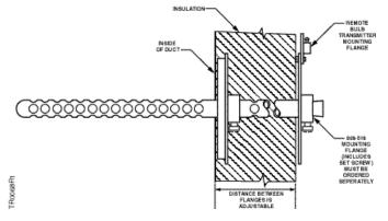
Figure 3. Mounting A Remote Bulb Transmitter on A Duct With Insulation on the Outside.
