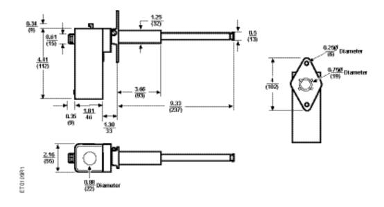
Figure 6. Dimensions in Inches (Millimeters in Parentheses).
