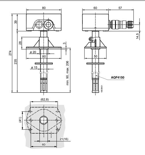
Drilling template with (without) mounting flange
