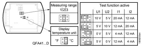
The setting elements are located inside the cover. A setting element consists of 6 pins and a jumper. It is used for selecting the required temperature measuring range and for activating the test function. Types with LCD display have a second setting element with 4 pins and a jumper.
