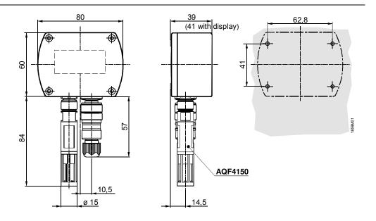
Dimensioning without (with) LCD-display Dimensions in mm
